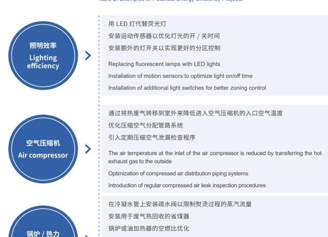
Installation of traps on condensate pipes to limit steam flow during the ironing
