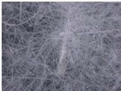
Figure B.1.4 Glue down: Down fibers and feather fibers twisted the root of the down cluster
