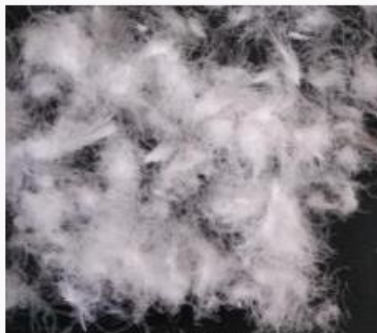
Figure A.1.3 Uneven down distribution, cotton shaped
