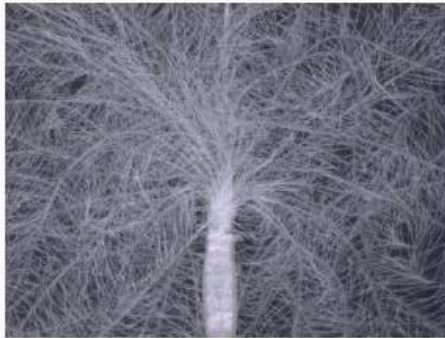
Figure B.1.1 Normal down: The core is clear and Down fibers emanating from the down core and showing a cluster in shape
