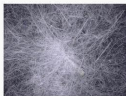
Figure B.1.5 Glue down: The core is not clear and has a reflective substance
