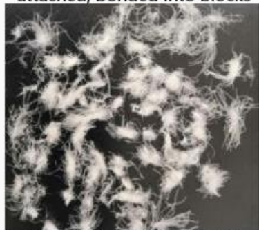
Figure. a. 1.4 Twisted down fibers and feather fibers, down cluster is not obvious
