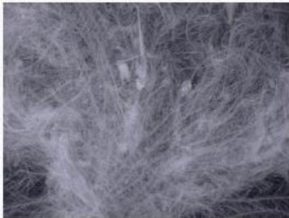
Figure B.1.2 Glue down: particulate matter scattered on down cluster
